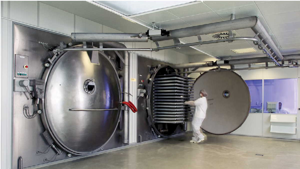
Photo: Freezer-dryer. Courtesy of Protifarm.
